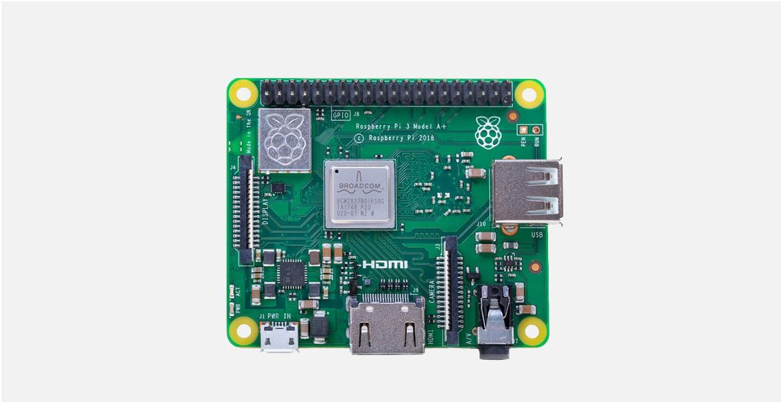
Raspberry Pi 3 Model A+, like Raspberry Pi 3 Model B+, has a 64-bit quad-core processor running at 1.4GHz, together with dual-band 2.4GHz and 5GHz wireless LAN, and Bluetooth 4.2/BLE. The dual-band wireless LAN comes with modular compliance certification.
